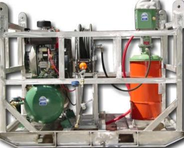
Climax Skid Mounted Lubrication System: Gas or Diesel Compressor
